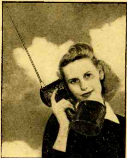
The pressure of a finger on a control switch permits the operator to "talk" or "receive."
